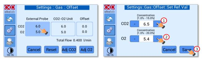
Figure 46. Manual Calibration (a – b).
